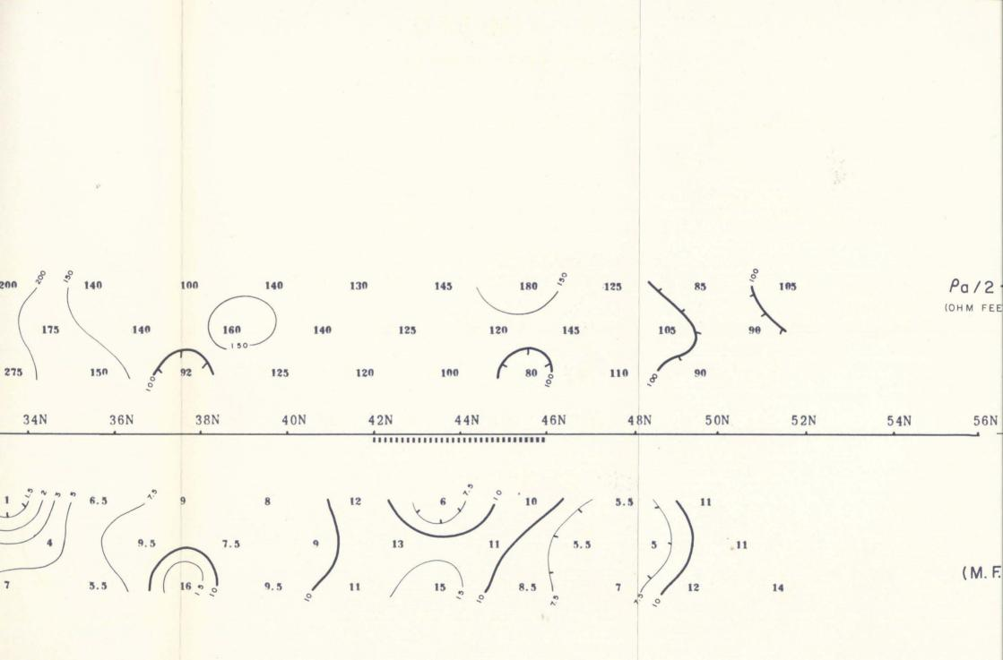
INDUCED POLARIZATION AND RESISTIVITY SURVEY
