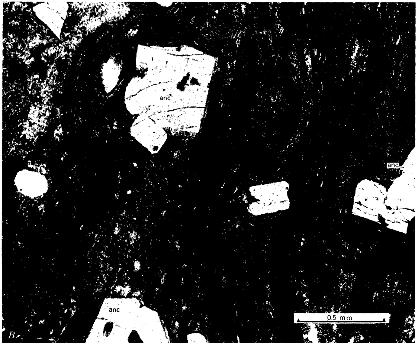
FIGURE 200.1.—Photomicrographs of thin sections of soda rhyolite intrusive, A , and flow-banded and autobrecciated flow, B . Phenocrysts of anorthoclase (anc) and diopsidic pyroxene (py) in fine-grained groundmass of quartz and alkali feldspar (light colored minerals) and acmite, riebeckite?, aenigmatite-rhönite?, and magnetite (dark colored minerals).
