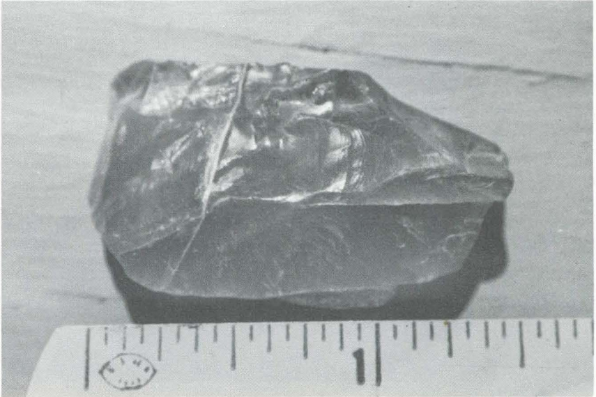
Figure 4. A large aventurine feldspar fragment (scale in inches) from the Oregon sunstone locality showing typical conchoidal fracture.
