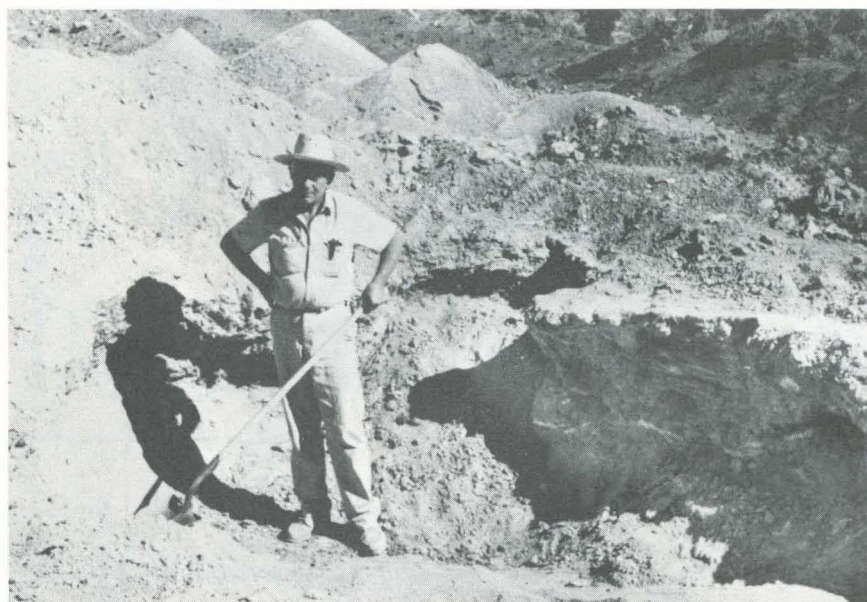
Figure 11. This view of a sunstone mining operation shows the inverted cone-shaped area of decomposed basalt. Note piles of screened debris in background.
