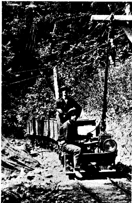
Figure 13. Electric tram that once ran between Musick mine and Champion mill. (Photo courtesy Ray Nelson)
