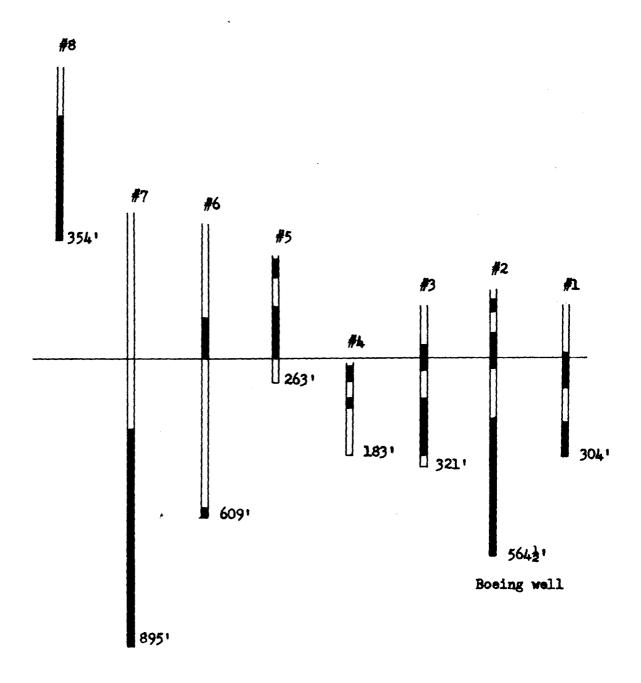
Figure 3. Reported basalt-sediment relationships at depth under the Boardman Bombing and Gunnery Range and area to the west thereof.
