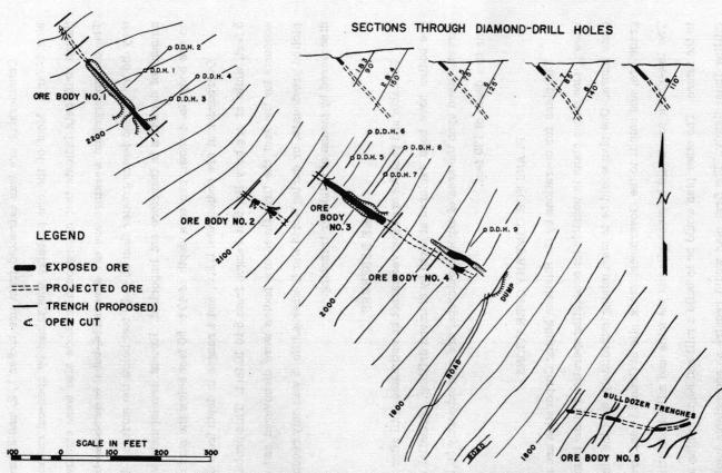
FIGURE I. PLAN AND SECTIONS, SOURDOUGH CHROMIUM MINE
