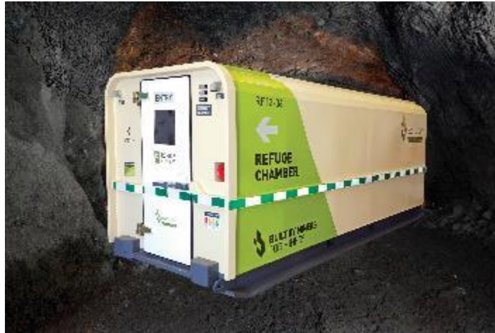
Figure 29. Typical Mobile Refuge Station
