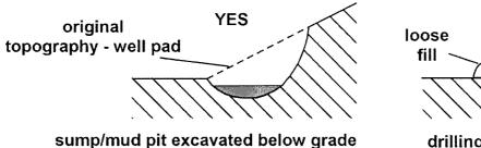
drilling fluids held by loose fill
