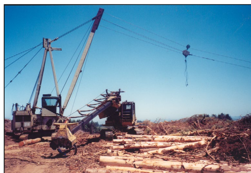
Figure 2.14: A yarder, which uses a system of cables to pull felled logs up to the landing where they can be processed for transport.
