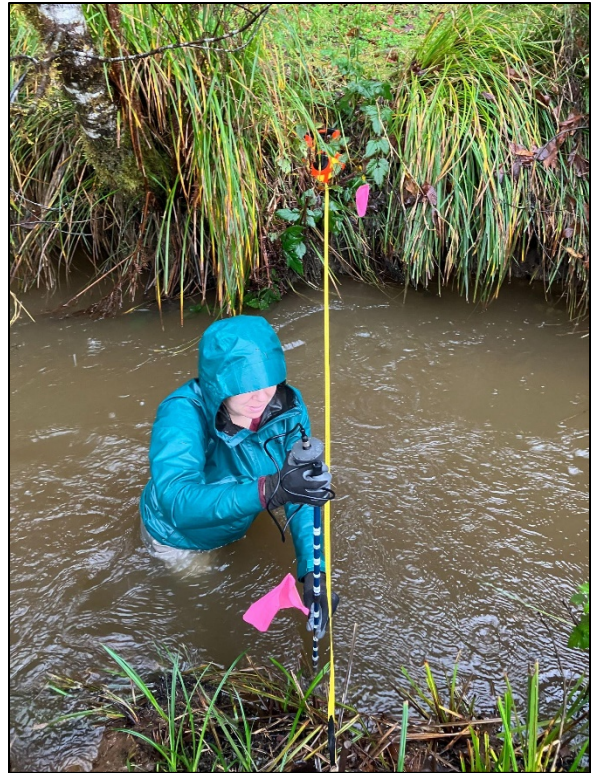
Figure 8. A surveyor measuring stream water velocity to quantify flow.
