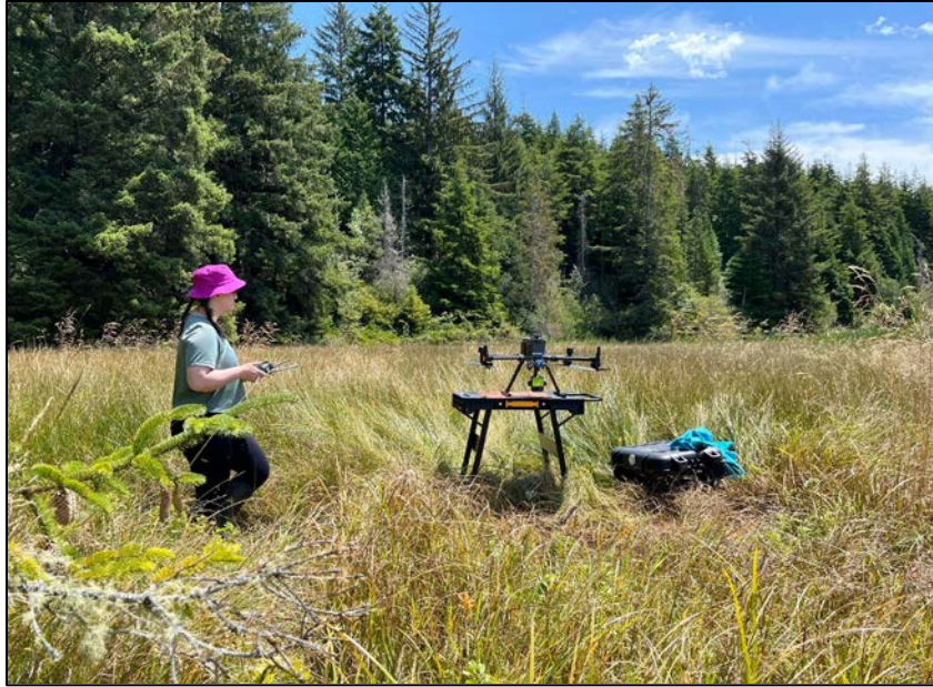
Figure 15. A field researcher conducting a UAS survey equipped with LIDAR and multispectral sensors at Toms Marsh.
