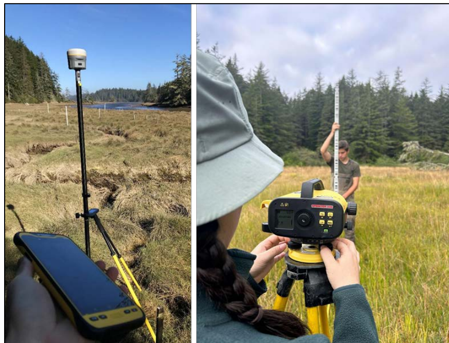
Figure 3. Field methods to determine elevation. At left, surveying with an RTK-GNSS rover, and at right, using a Sprinter level.
