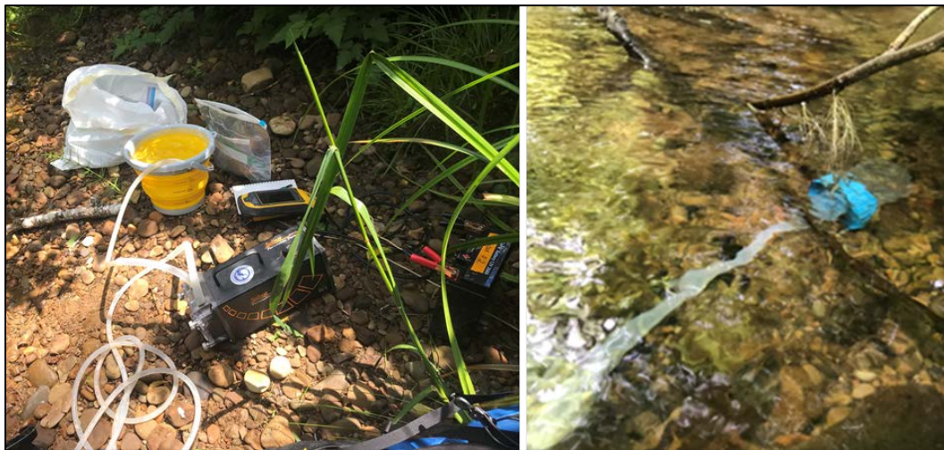
Figure 18. eDNA sampling kit setup (left) to collect filtered water samples from a stream (right).
