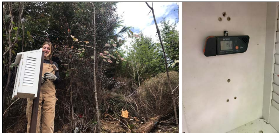
Figure 12. Thermometer shelter used to measure forest microclimate conditions.
