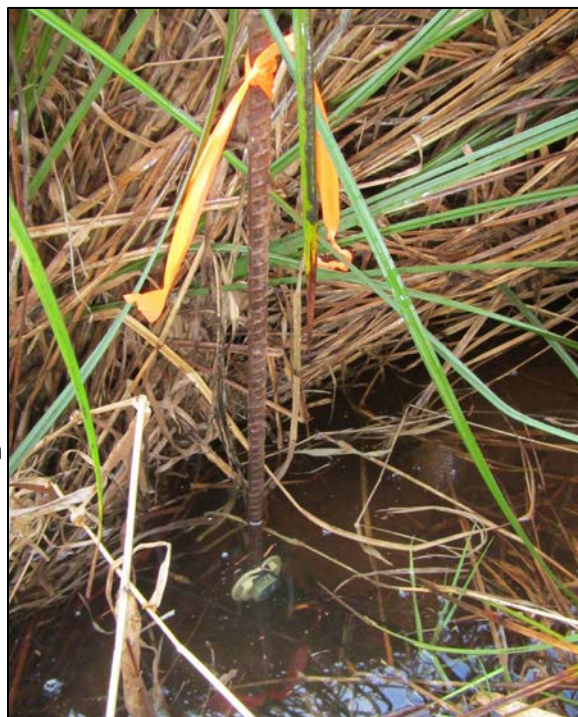
Figure 6. Example of stream temperature monitoring. The temperature sensor is located approximately 10 cm above the creek bed.
