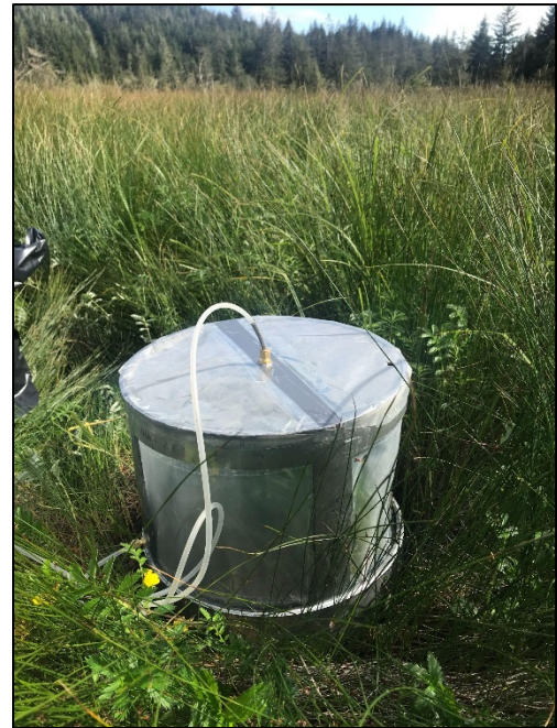
Figure 11. A closed-loop chamber used to measure GHG concentrations in FSM.
