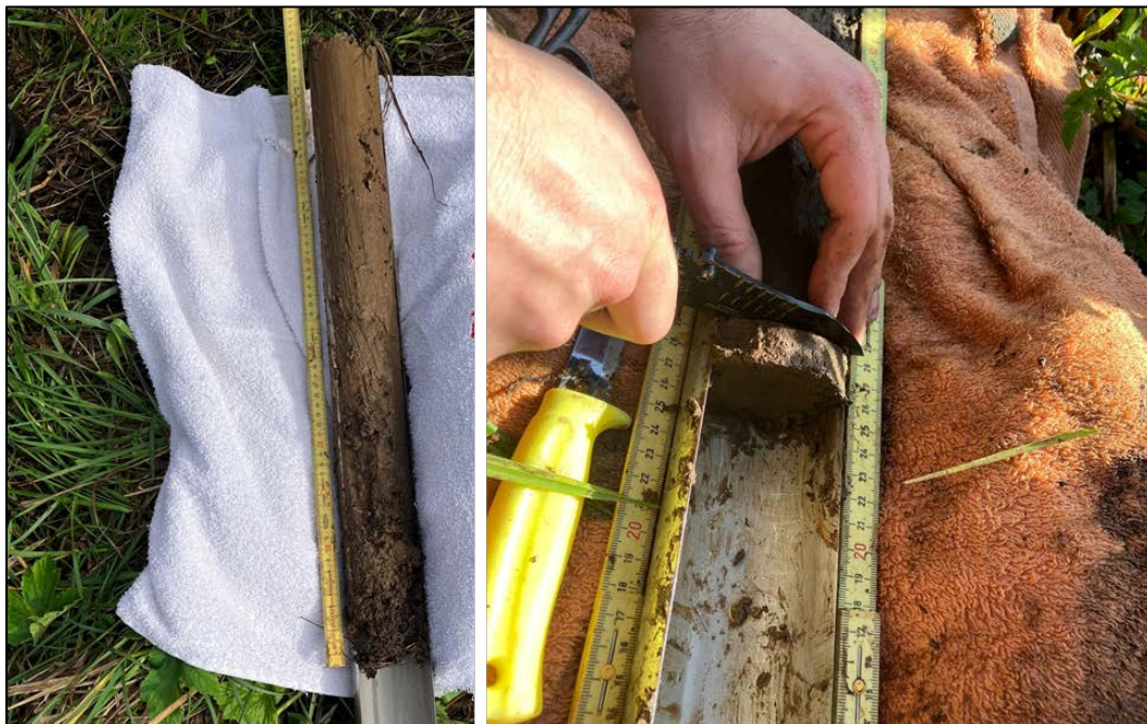
Figure 9. Example soil core collection to determine soil characteristics including dry bulk density, carbon content, and accretion rate.
