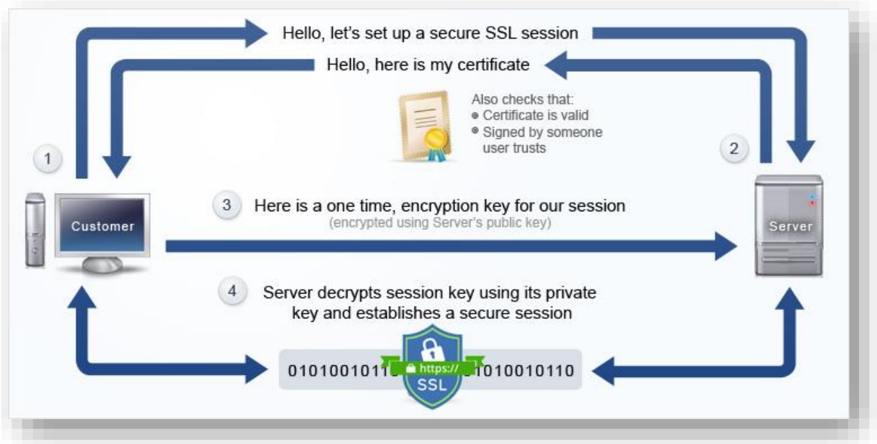
Figure 3: How TLS works
