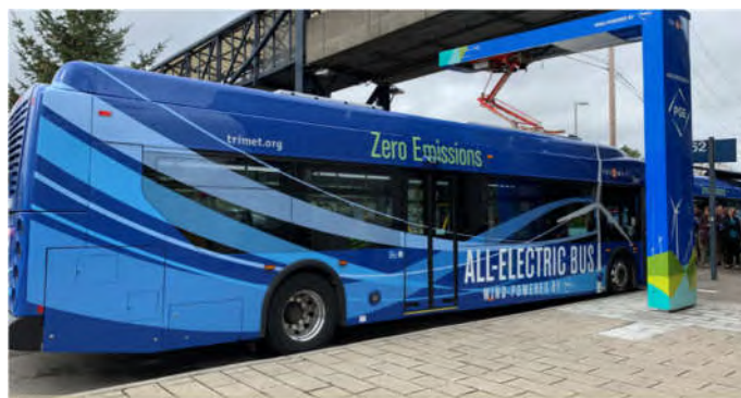
An all-electric TriMet bus recharges at the Sunset Transit Station in Hillsboro.
