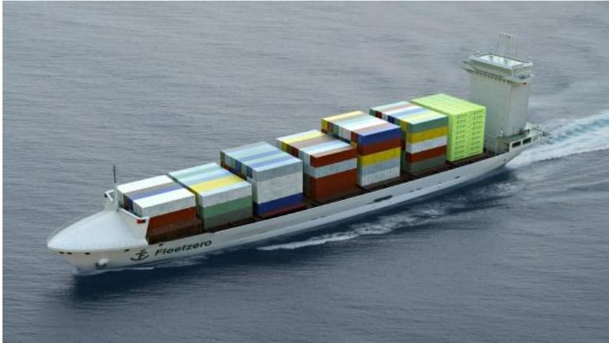
piloting electrification, and a startup named FleetZero is designing smaller cargo ships while rethinking the way cargo is moved around the globe to make electric ships more feasible.<sup>23</sup> This includes storing batteries in containers so that they can easily be picked up and swapped out when in port. However, overall battery electric alone is likely not sufficient to meet most ocean craft needs.
