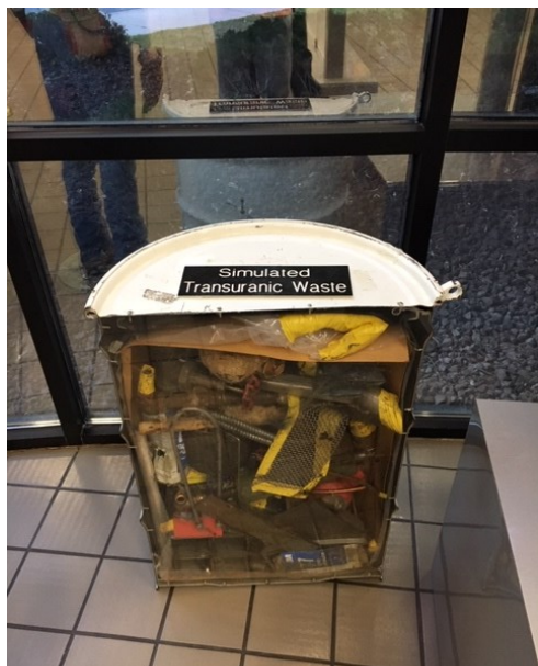
TRU container with contaminated equipment.
