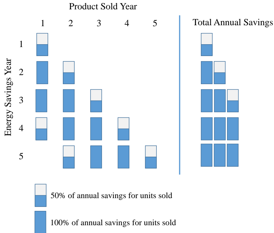
Figure 1: Generic example of calculated savings for a product with a 3 year lifespan, adopting a recommended standard over a period of 5 years. Total cumulative savings over the 5 year period is 10.5 times the annual purchased product savings.
