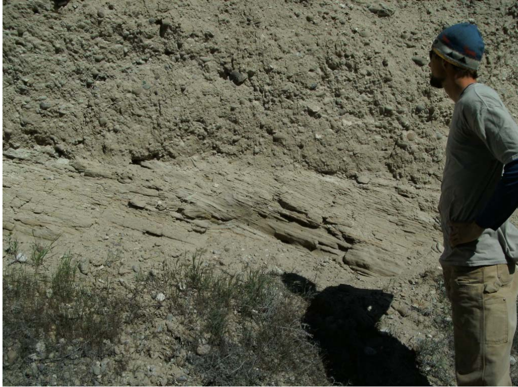
Typical exposure of the Dalles Formation, which consists of weakly cemented, gravelly sand to gravel and thinly bedded, very weak sandstone and siltstone.
