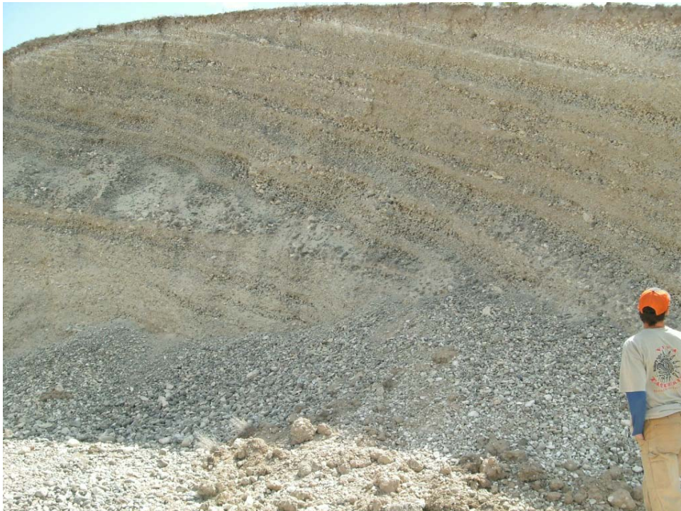
Exposure of catastrophic flood deposits in a gravel pit near Montague Lane. The bedding dips west (toward the right side of the photo) which indicates a westward flow of floodwaters. Deposits consist of matrix-free layers of poorly graded, fine gravels to small cobbles separated by gravelly sand to sandy gravel layers. Note the lack of loess deposits. Exposure is approximately 25 feet high.
