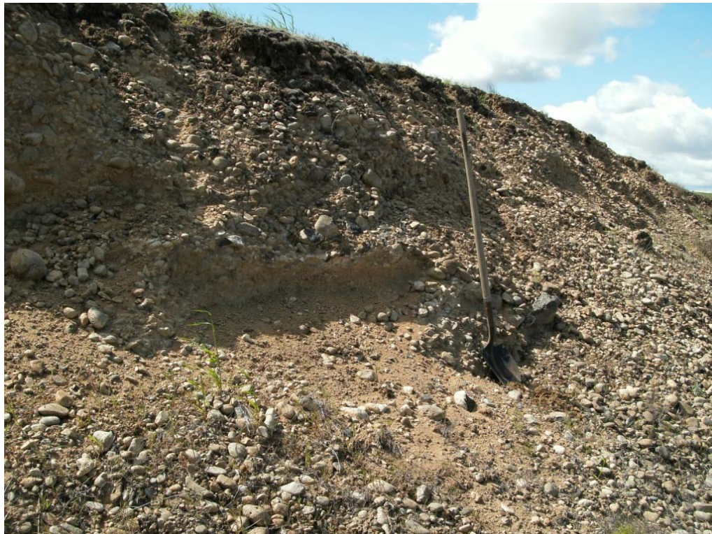
Exposure of the Dalles Formation along Montague Lane. The formation consists of weakly cemented, gravelly sand to sandy gravel with caliche layers. Note the absence of silty loess cover at this location.
