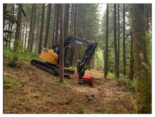
Figure 23. SlashBuster Clearing Right of Way
