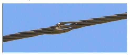
Figure 29. Damaged Conductor Identified by EFD System
