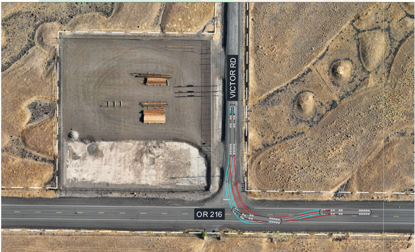
High Resolution Image & Turn Simulation for OR-216 to Walters Rd
