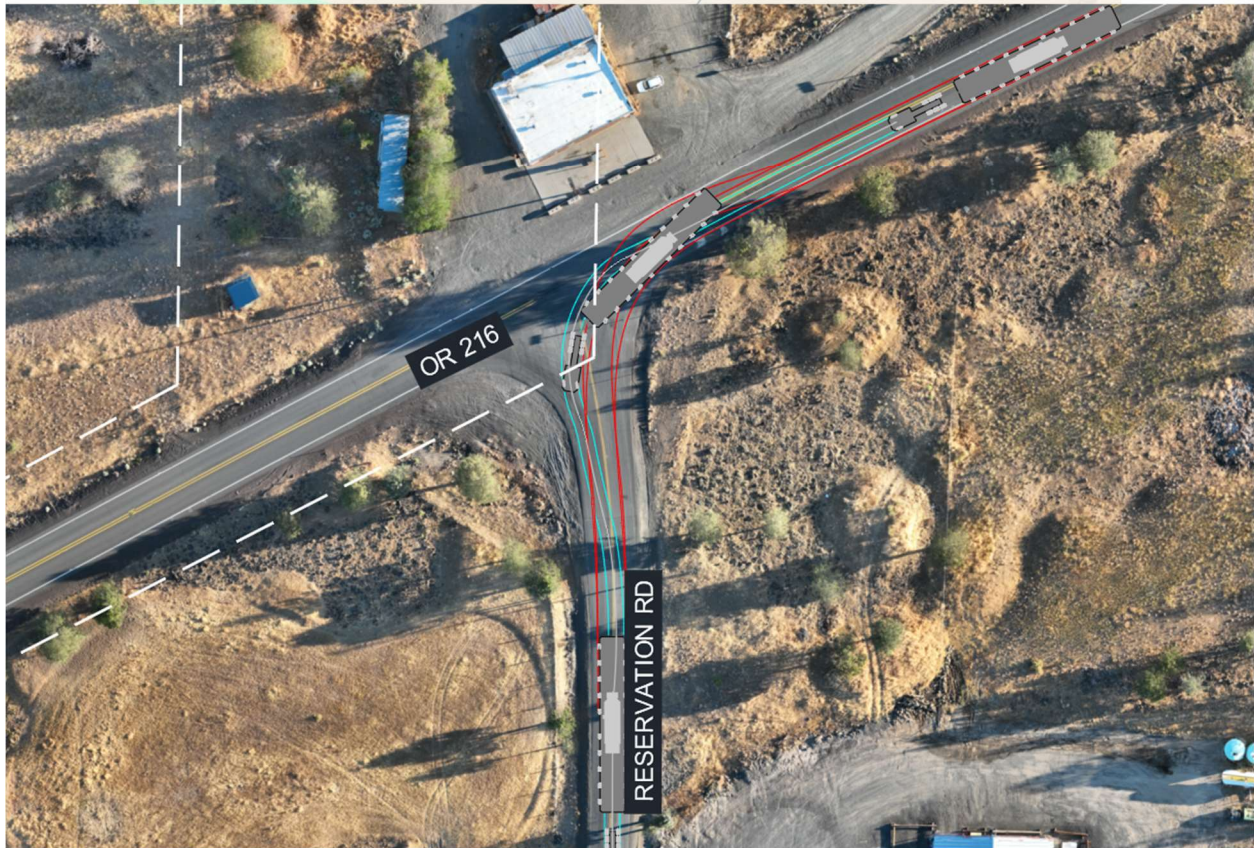
High Resolution Image & Turn Simulation for OR-216 to Reservation Rd
