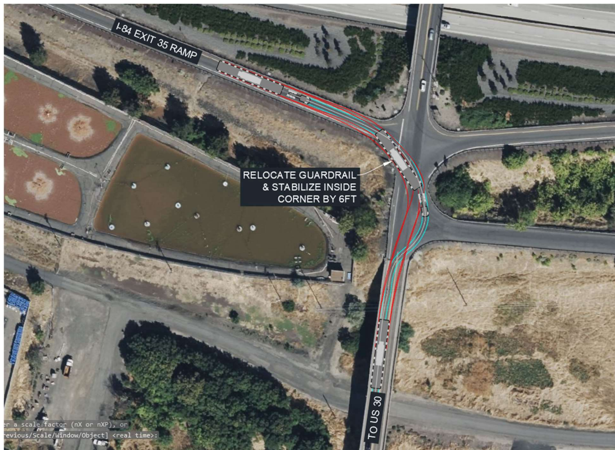
Exit 35 Interchange – Transformer Vehicle Turn Simulation (Recommended Bypass)
