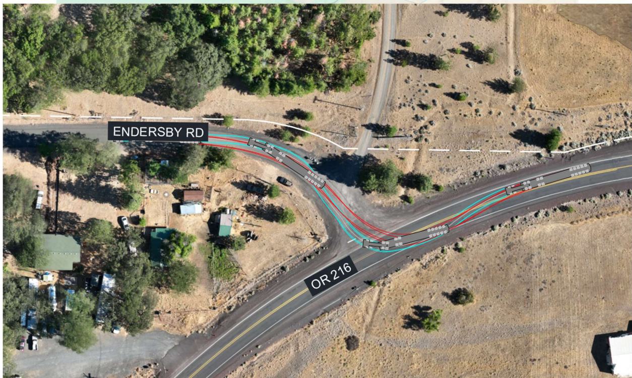
High Resolution Image & Turn Simulation for OR 216 to Endersby Rd
