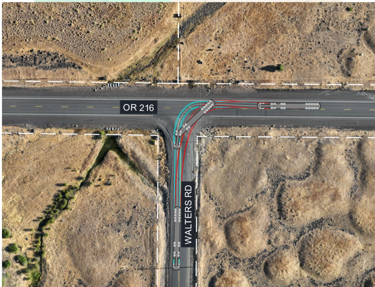
High Resolution Image & Turn Simulation for OR-216 to Walters Rd
