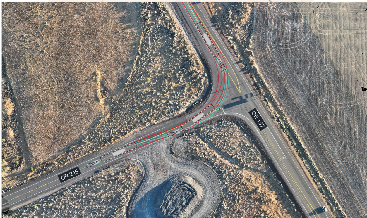
High Resolution Image & Turn Simulation for OR-197 to OR-216
