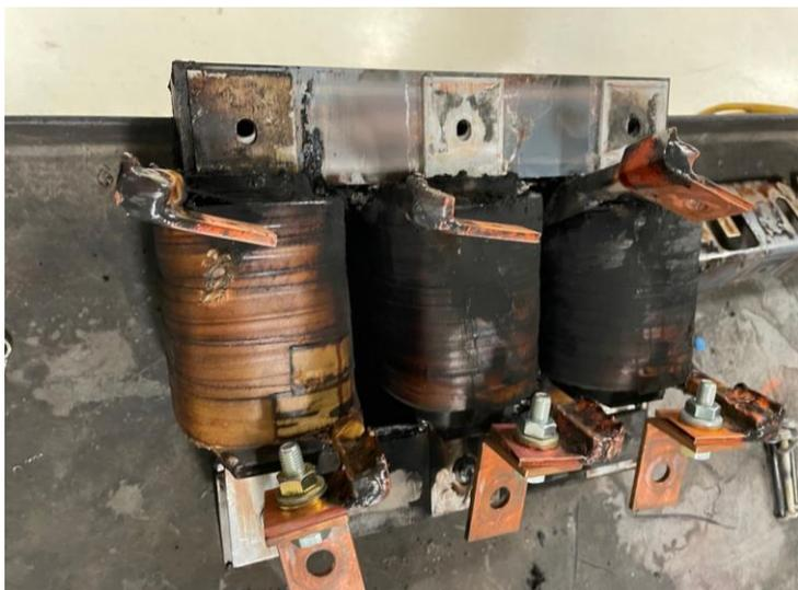
Damaged startup heater inductor
