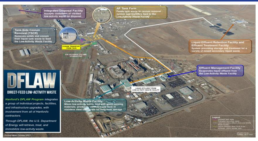
**DFLAW** is an assembly of highly interdependent projects and infrastructure improvements, managed as a program, that is operating together to vitrify and dispose of low-activity waste.
