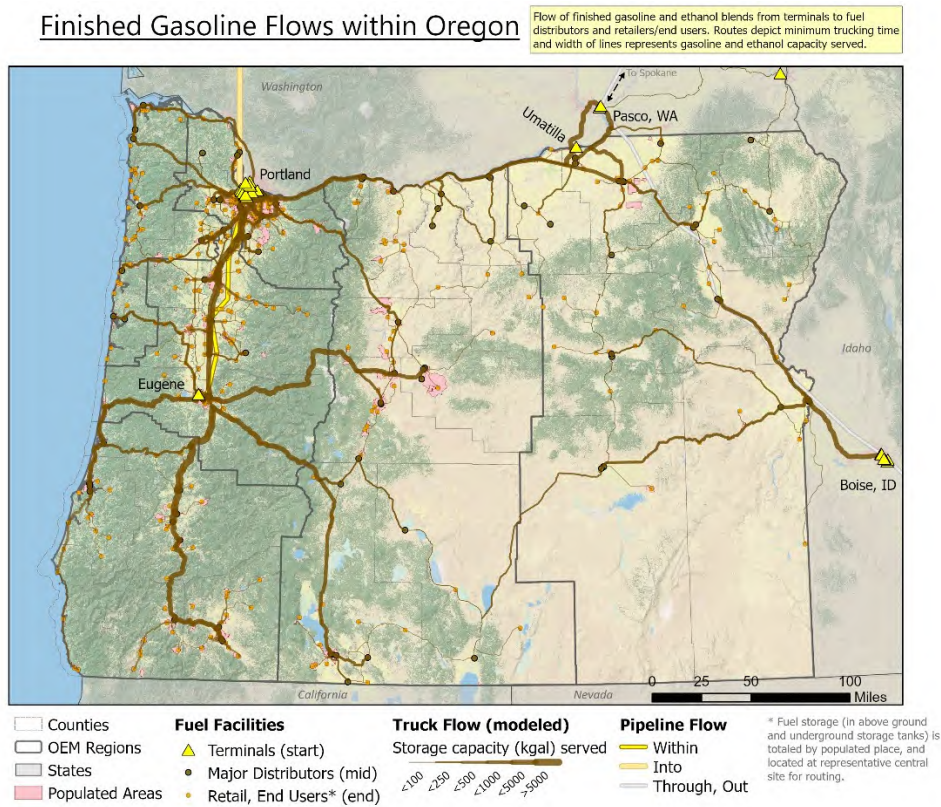
Figure 35: Flow of Finished Gasoline from Terminals to Fuel Distributors and Retailers/End Users Within Oregon 36–38,48–51
