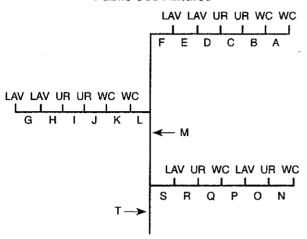
In the example below, fixture units assigned to each section of pipe are computed as follows: Note: Each capital letter refers to the section of pipe above it, unless otherwise shown.
