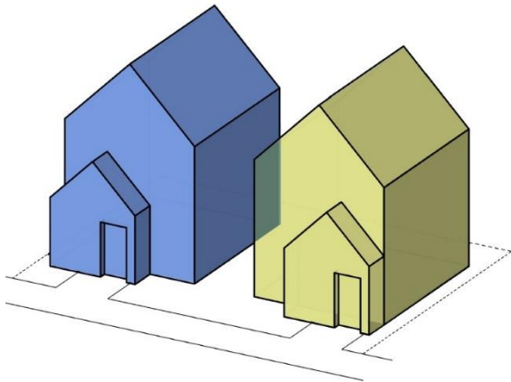
Figure 7. Detached Duplex Units Side-by-Side
