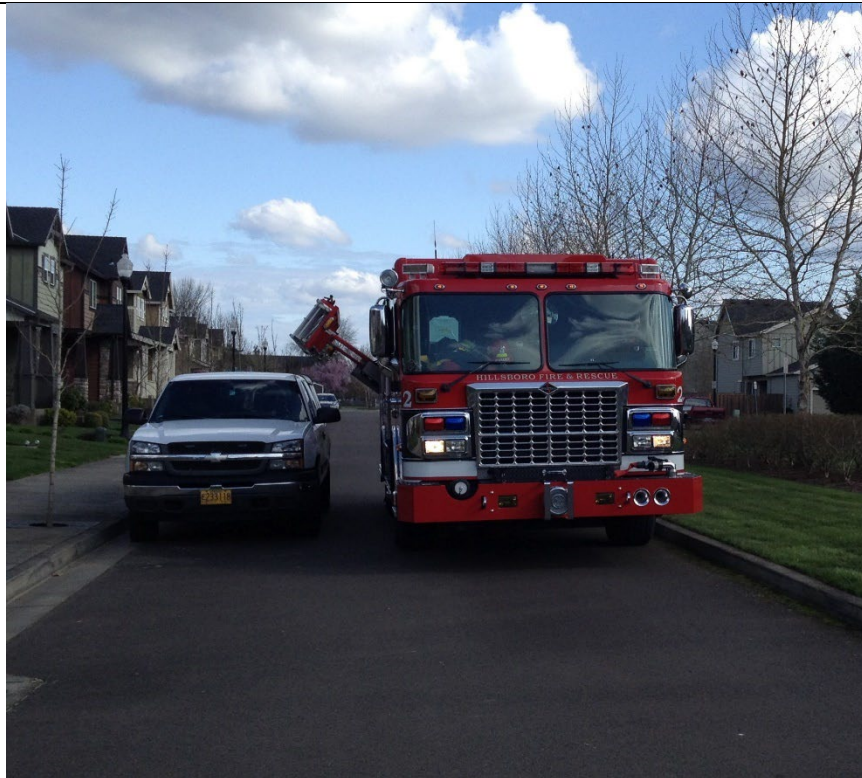
Figure E4: How On-Street Parking on Narrow Pavement Prevents Emergency Responders Accessibility to Ladder
