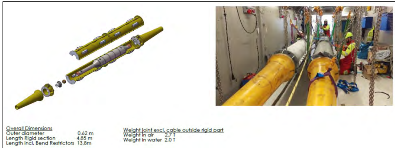
Figure 15: Undersea Power Cable Repair Joint (source: NKT)
