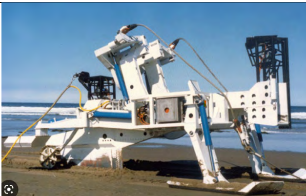
Fiber optic cable plow (source: submarinenetworks.com )
