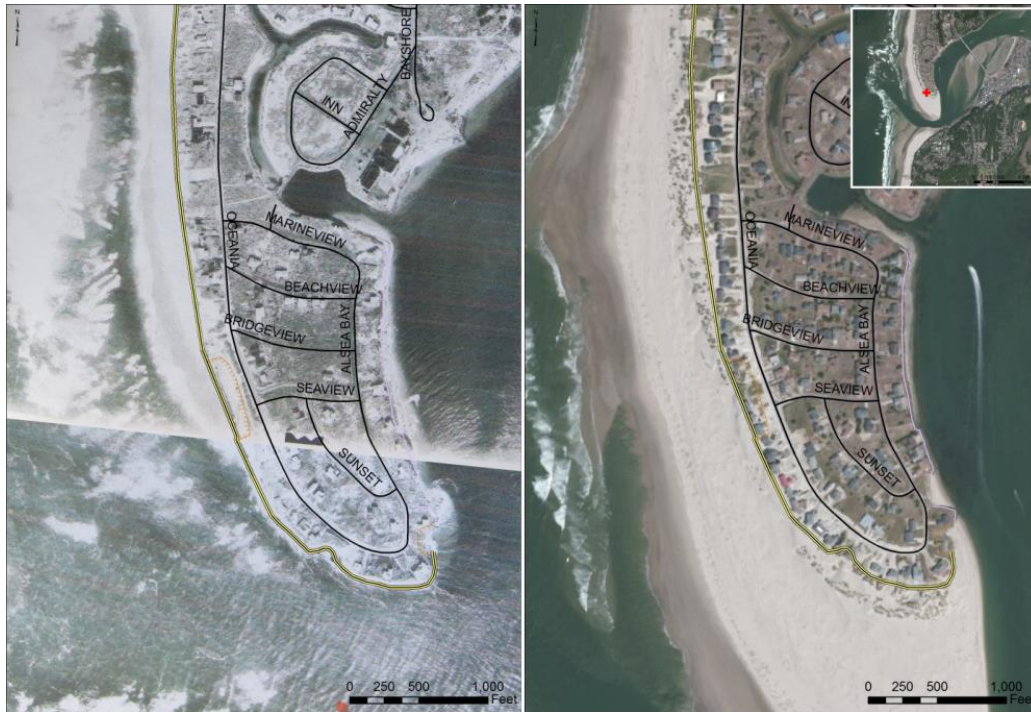
Figure 2-36. Alsea Bay Spit Erosion as a Result of the 1982-83 El Niño (left), and State of the Beach in 2009 (right)
