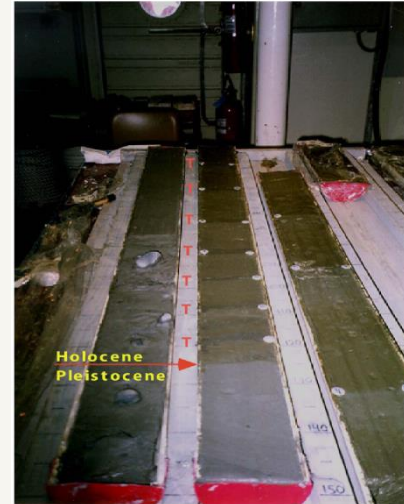
Figure 2-47. Deep Sea Sediment Cores that Record Past Megathrust Earthquakes off the Oregon Coast
