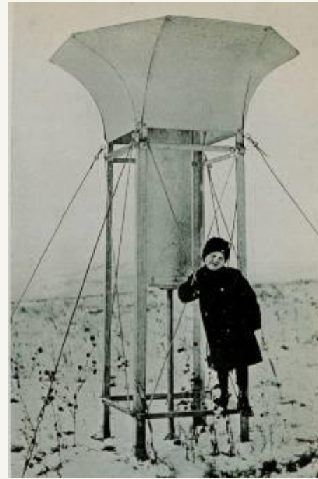
Figure 2-107. Shielded Snow Gauge Used in the Pacific Northwest to Register Snowfall, 1917
