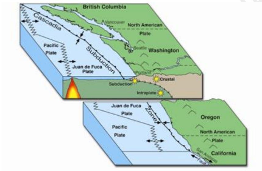
Figure 3.3.3-4: General Source Areas for Subduction Zone, Crustal Earthquakes, and Intraplate Earthquakes
