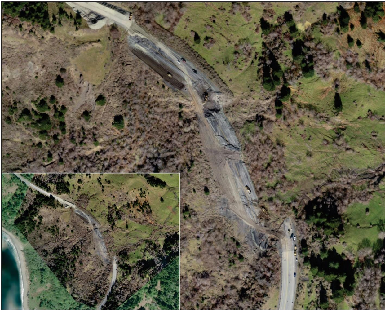
Figure 3.3.1-10: Landslide Movement Affecting U.S. Highway 101 at Hooskanaden Creek on March 3, 2019
