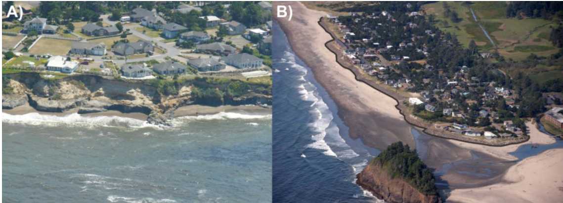
Figure 3.3.1-4 (A) Houses Line the Cliff at Fogarty Creek in Lincoln County. (B) Extensive Erosion along the Dune-Backed Beaches in Neskowin Have Resulted in the Construction of Massive Riprap
