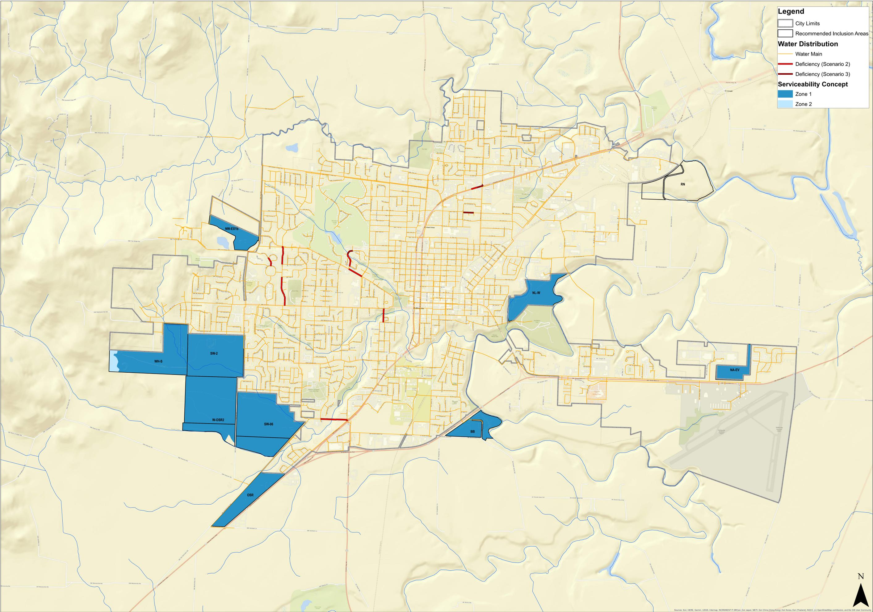
Map reflects study areas and concepts, as of 10/8/2020. Deficient pipes are identified when flagged under Scenario 2 (PZ1, west of river) and under Scenario 3 (PZ1, west/east). See TM for details and results.
