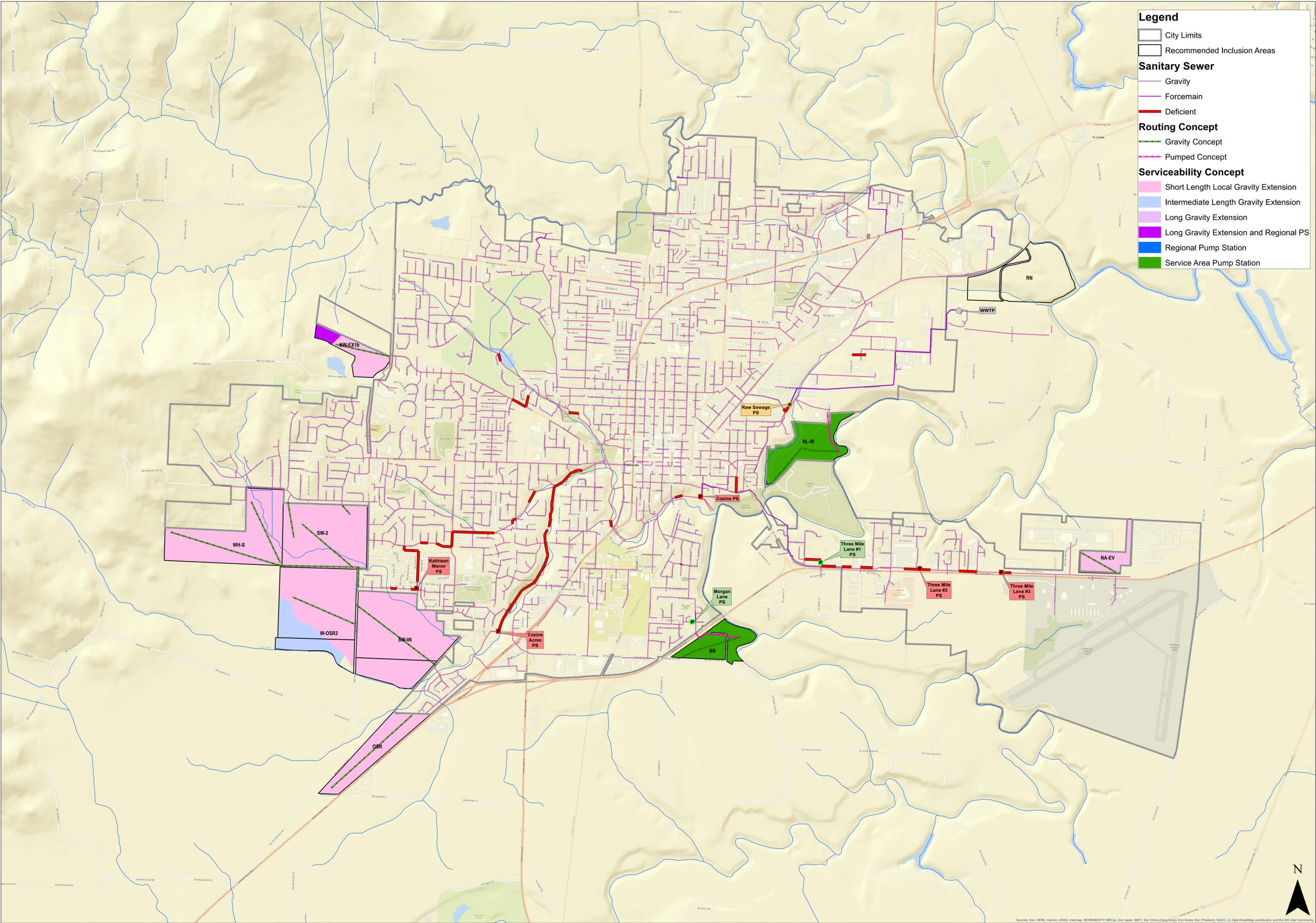
Map reflects study areas and concepts, as of 10/8/2020. Call-outs identify pump stations & pipes identified as deficient with color-coding (red, orange). See TM for results.
