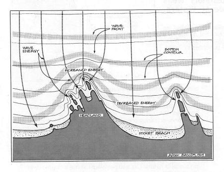
Figure 19. Wave Refraction
