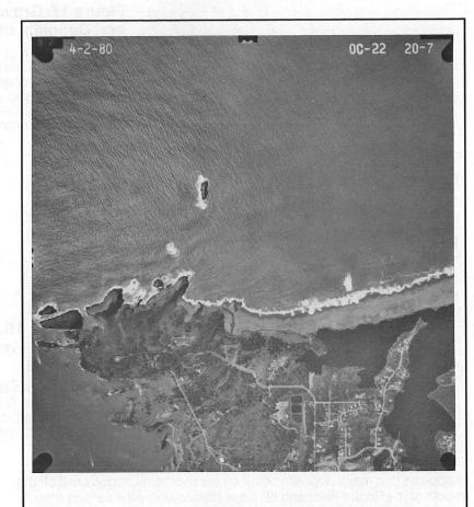
Figure 20. Aerial View of Wave Refraction Around Offshore Rocks
