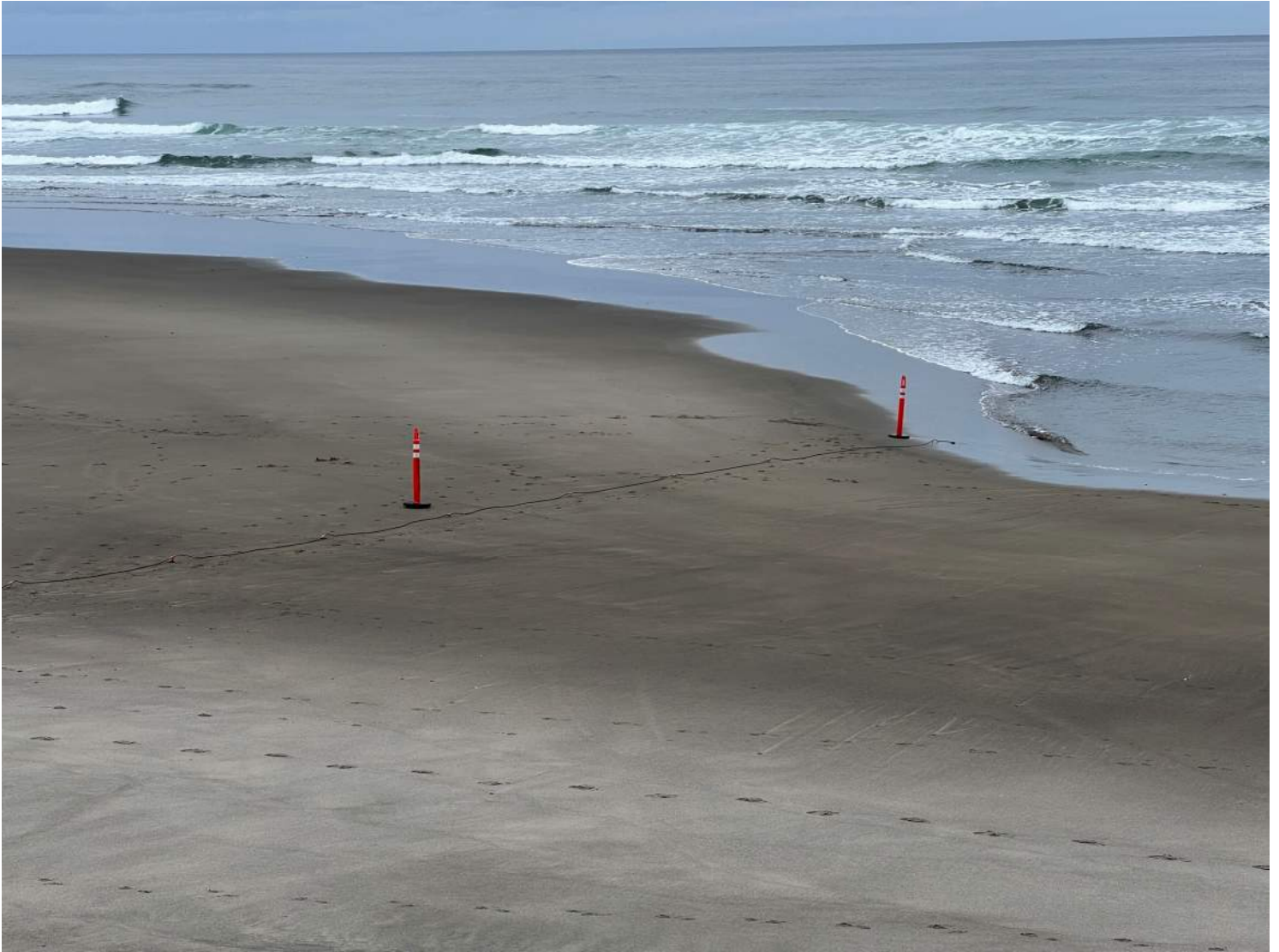
ERT test set up on the beach
