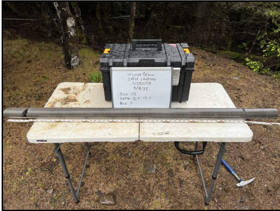
PHOTO 25: BORING B-1, CORE RUNE 13: 126.5 FT -131.5 FT
