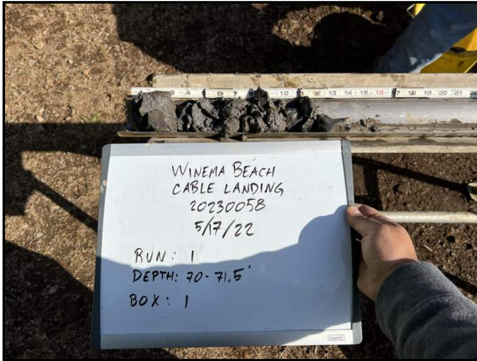
PHOTO 13: BORING B-1, CORE RUNE 1: 70 FT -71.5 FT
