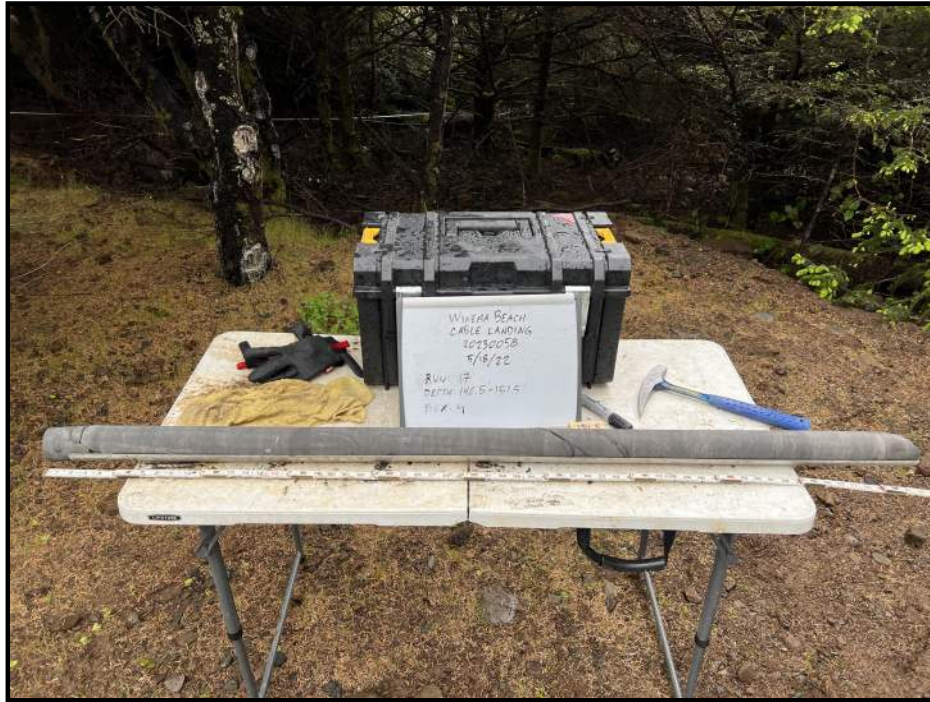
PHOTO 29: BORING B-1, CORE RUNE 17: 146.5 FT -151.5 FT
