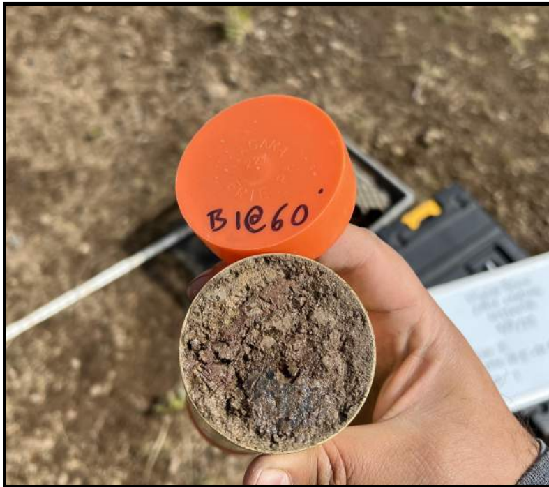
PHOTO 11: BORING B-1, 60 FT SAMPLE
