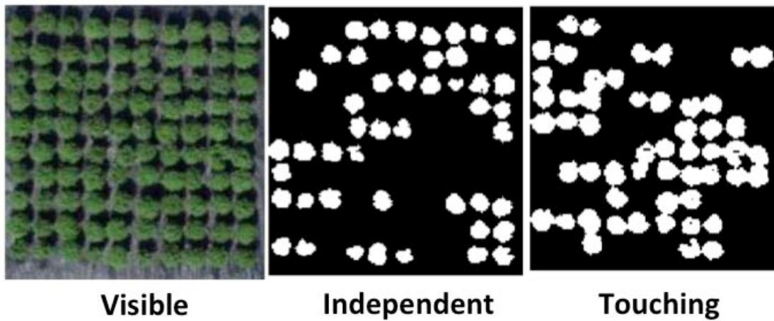
Visualization of new algorithm created by the University of Florida using green index and counting plants if not touching (independent) and canopy when touching (touching) separately resulting in 95% accurate inventory estimation.
