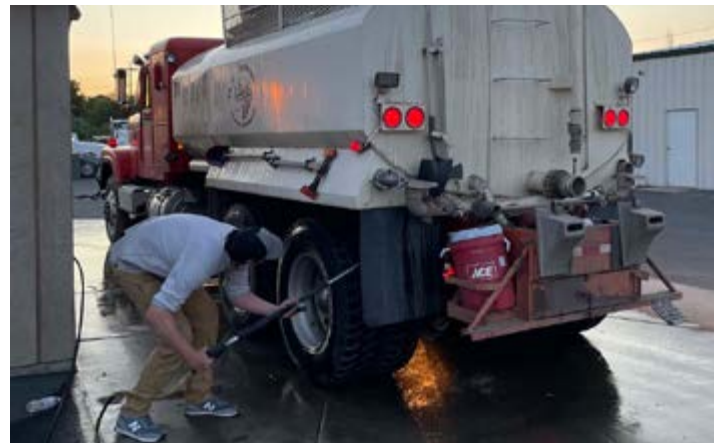
Equipment Wash Station, crews wash vehicles to prevent spreading noxious weeds when entering and leaving fire zones.
