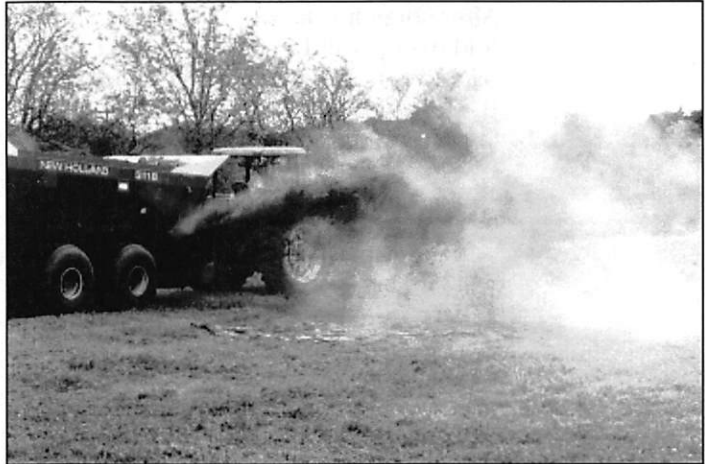
Figure 4. Place a tarp or piece of plastic in the field and apply solids over the area.
