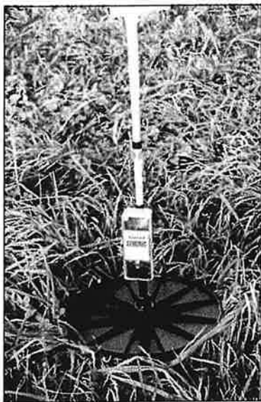
Figure 2.—The electronic rising plate meter estimates standing forage dry matter, accounting for pasture height and density.
