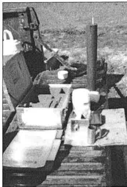
On-farm quick tests determine manure N content within a few minutes.
