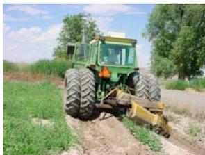
All the farmer has to do is create two deep furrows at the end of the field using a terracing blade.
