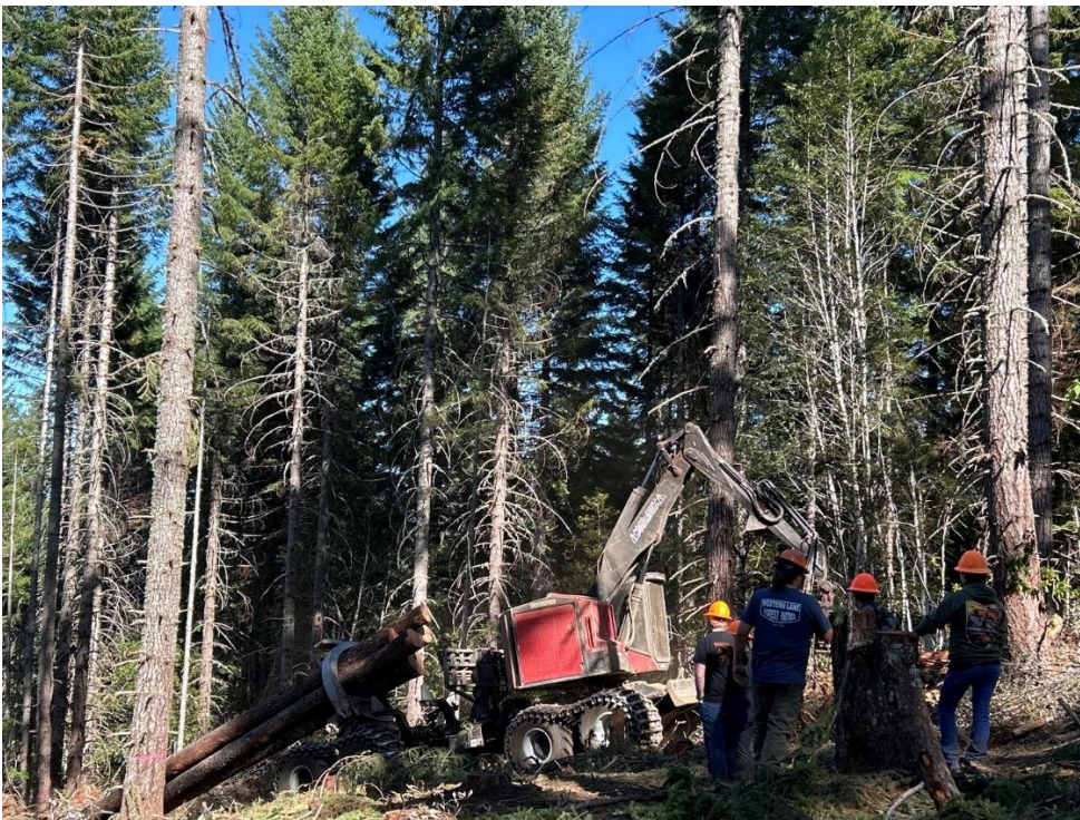
Coos Unit staff checking out the TimberPro TF840D in action for ground-based felling/yarding
