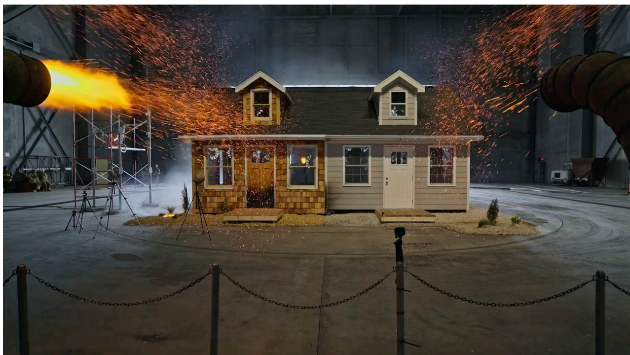
Figure 4. Testing resistance of home building and landscaping materials to ignition from wind-blown embers. Photograph courtesy of ElementalFilm.com.
