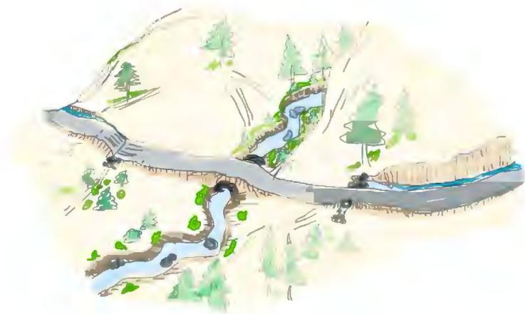
**Fill failures and diversion of water crossings can cause fluvial hillslope erosion.**
