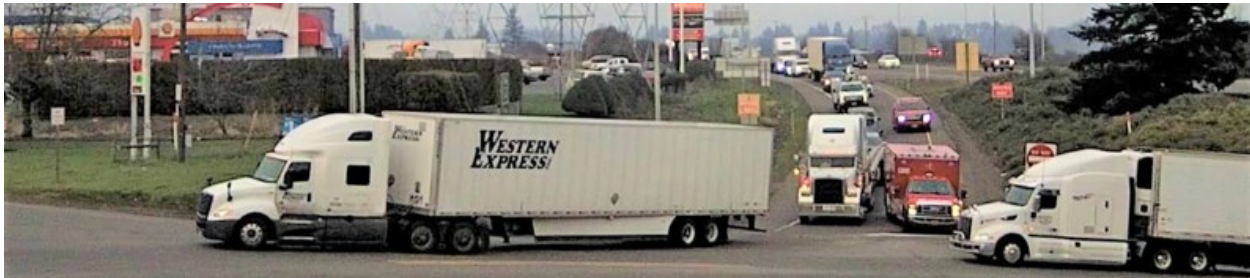
SB Exit Ramp: Vehicles form two lanes, driving on shoulder of single lane exit ramp.
