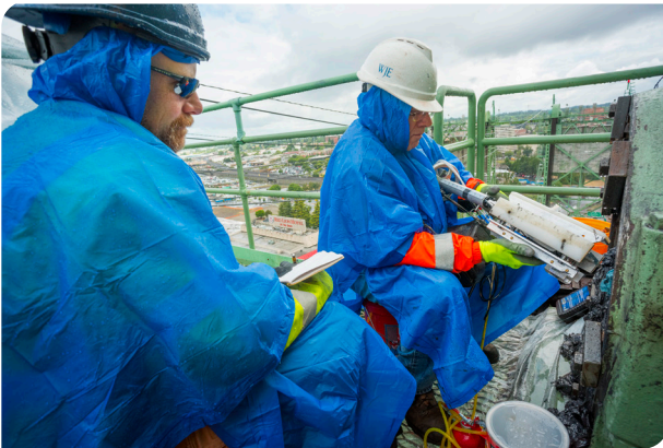
Monitoring a crack in the trunnion of the Interstate Bridge using UT.
