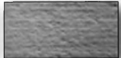
CSP 4 (light scarification)
