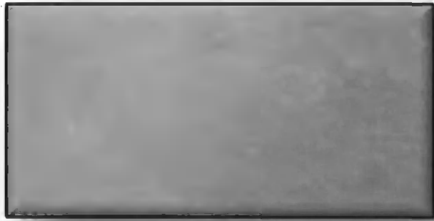
CSP 1 (acid etched)
