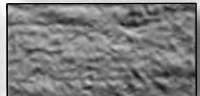
CSP 6 (medium scarification)
