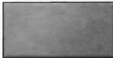
CSP 1 (acid etched)
