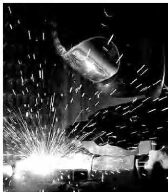
Figure 10-44. Gas metal arc welding process.
