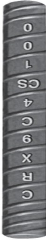
Bars #3 through #9 (#3 through #6 coiled)
