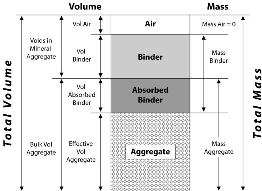
Each of the properties in the asphalt mixture phase diagram can be measured or calculated. For example: The mass of the aggregate is measured; the voids in mineral aggregate (VMA) is calculated; total asphalt binder can be measured but the amount available to act as a binder in the mix must be calculated because it is the quantity left after the aggregate has absorbed some of the asphalt binder.
