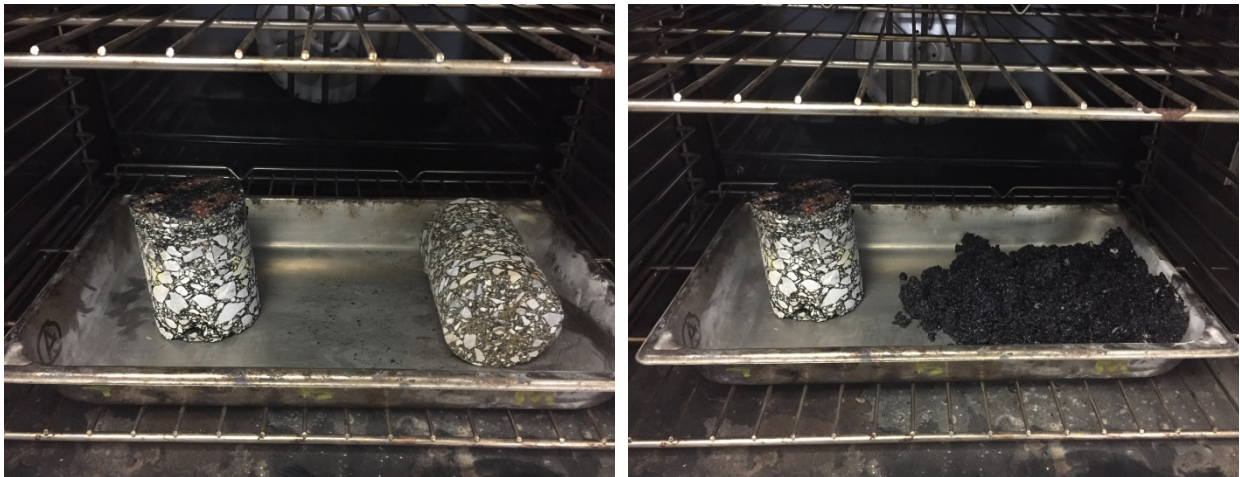
(a) 30 min after oven storage at 230°F
