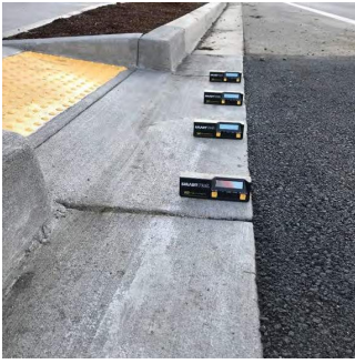
Measuring Counter Slope with a 6-inch Level
