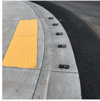
Measuring Counter Slope with a 6-inch Level
