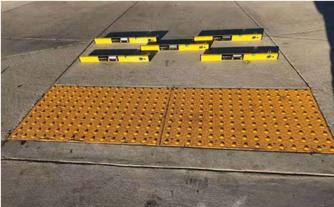
Example of Cross Slope Level Placement on a Ramp Run
