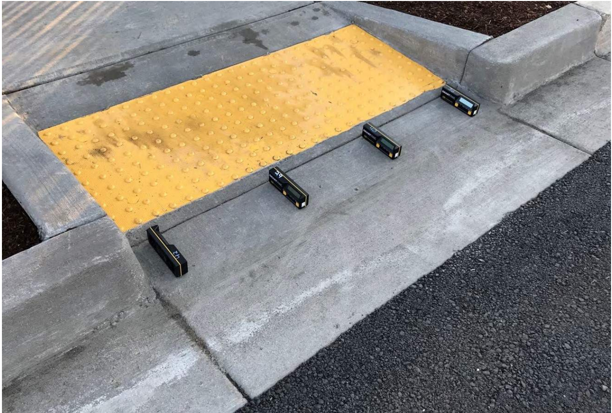
How to Measure Curb Running Slope
