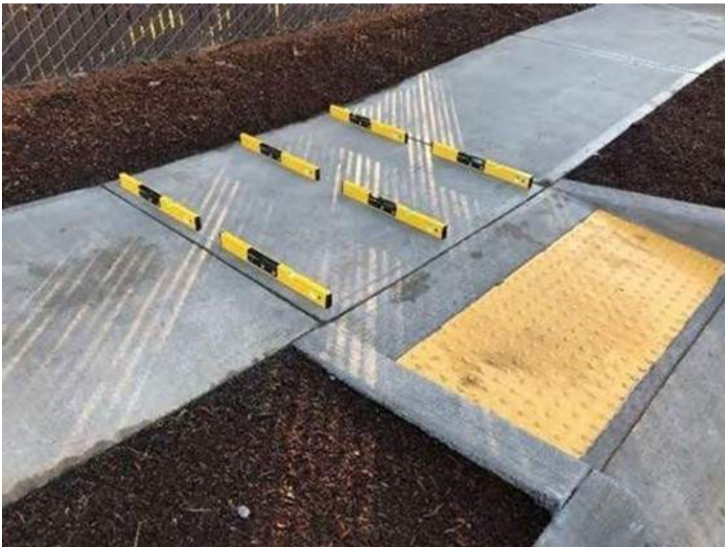
Measuring Slopes in the Y Direction on a Combination Curb Ramp
