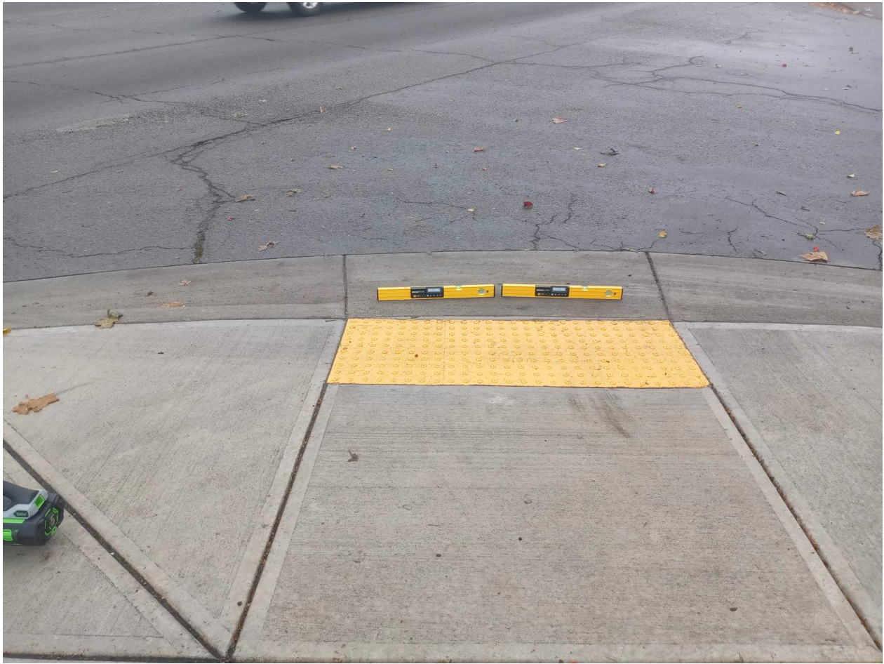
How to Measure Gutter Flow Slope
