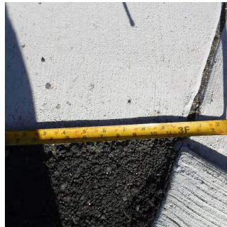
5.0 feet Between Ramp Runs Photo 1-2: A close up of the measurement "5.0 feet Between Ramp Runs Photo 1-2" showing that the length is 3.0 feet. Measurement for 5.0 feet between ramp runs is taken at the back of walk.
