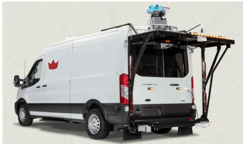
Figure 4 – Pavement Data Collection Vehicle used for Automated Distress Survey
