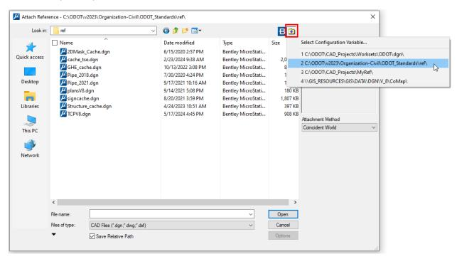
The top location (1) in the shortcut list is always the directory of the open DGN file. Standard cache files can be accessed by using the shortcut that ends with **ODOT\_Standards\ref\**. Personal references can be easily accessed from the shortcut that ends with **CAD\_Projects\MyRef\** - and of course, that will show any files that you place in that location on your computer.
